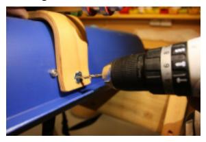
2. Remove the wheel support and enlarge the holes in the pulk using a M6.5 drill bit.
