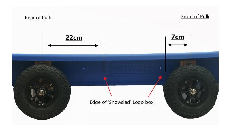
The suggested mounting position for the Pulk wheels is shown in the above diagram.
